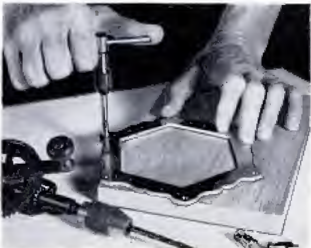
Above, brass is painted with India ink and the outline of the trivet frame is scribed on the brass, using a cardboard template. Holes for the finials are center-punched, drilled and then tapped, as below
